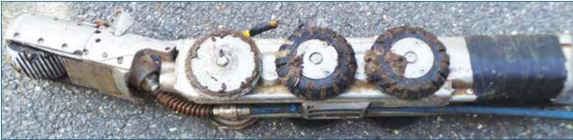
A close-up of the CCTV camera used for the sewer lateral inspection, as soon as it came out of the manhole
